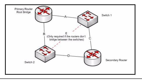
If the primary router fails, the secondary router becomes both the active router and the root bridge, and traffic from the switches flows on the reconfigured spanning tree along links C & D. If bridge priorities are not managed, traffic from one switch may be directed through the secondary router and the other switch as normal operation.
